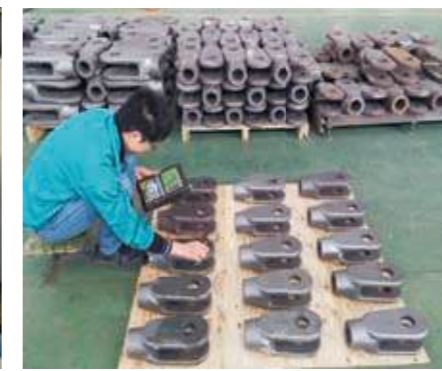
Ultrasonic Flaw inspection
