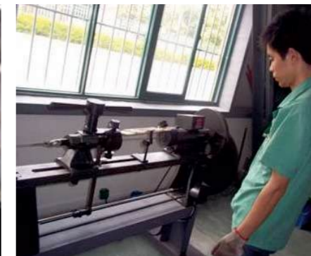
Torsion Testing for Steel Wire
